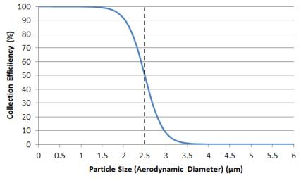
Figure 3 — Indicative Size-Selection Curve for a PM<sub>2.5</sub> Inlet
